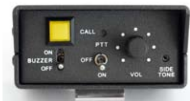
BP-100 portable 1 channel intercom-station (Belt-Pack)
